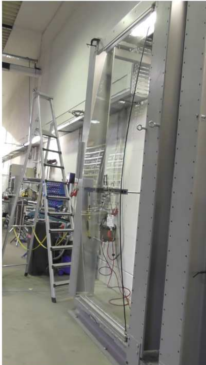
Line Load test with glass (5-0,76-5)
